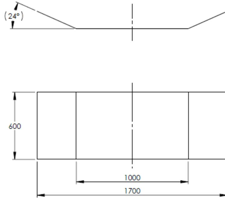
**Figure 5. Bumper Cladding**
