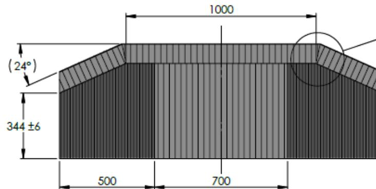
**Figure 3. Base Plate and Mounting Flanges**
