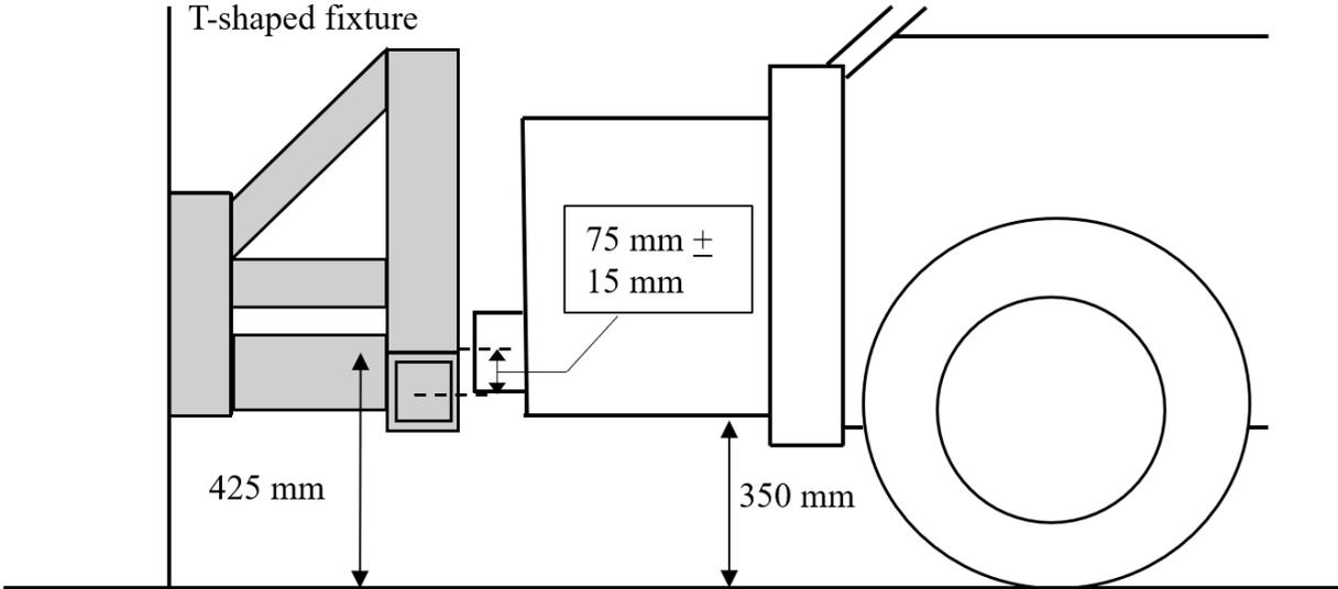
Figure 1B. Lateral barrier alignment
