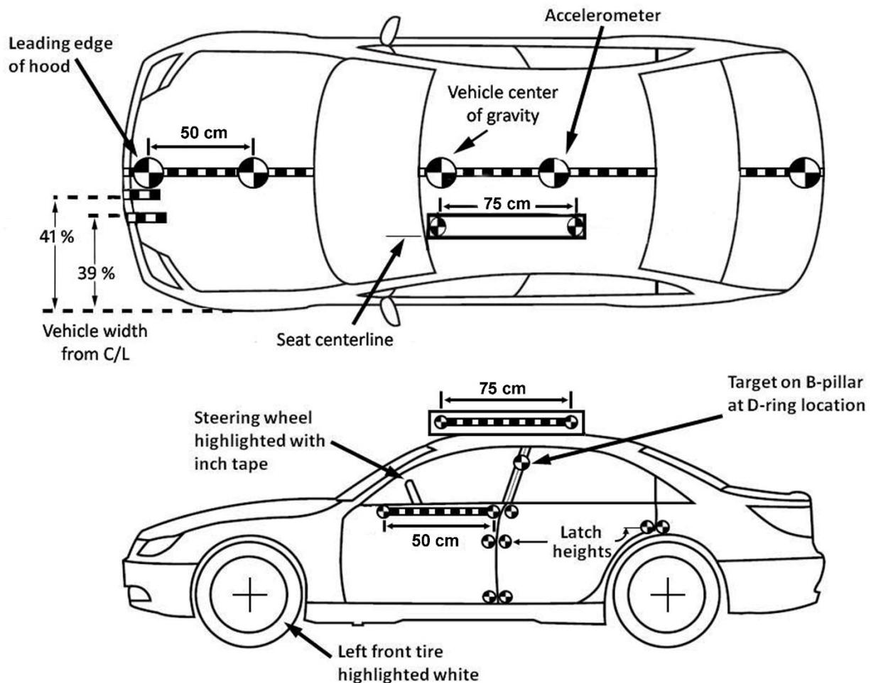
The driver's head restraint (if adjustable) is adjusted upward until the top of the head restraint is level with the top of the dummy's head. If the head restraint lacks sufficient height adjustment to reach the top of the dummy's head, the test is conducted with the head restraint set at its highest setting. The locking
