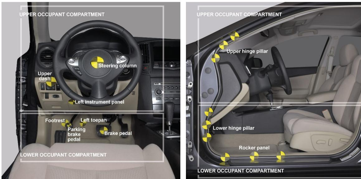
**Left instrument panel (one point):** The left instrument panel lateral coordinate is defined by subtracting 15 cm from the steering column reference lateral coordinate. The vertical coordinate is defined as 45 cm above the height of the floor (without floor mats). If the panel loosens or breaks away in the crash, the postcrash measurements are taken by pressing and holding the panel against the underlying structure.
