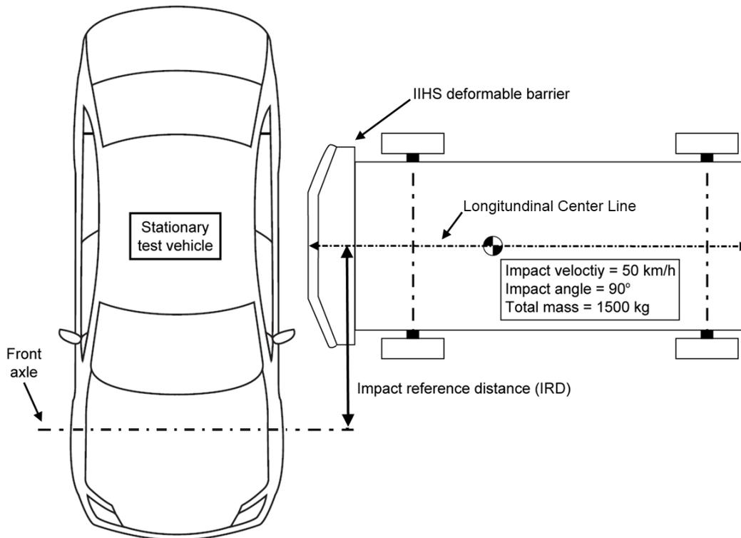
alignment may be modified to prevent direct loading to these structures early in the crash. To date, only one such vehicle has been tested by IIHS, the Smart Fortwo (188 cm wheelbase). Currently, there is no set alignment rule for vehicles that fall into this category, therefore impact alignment will be determined on a case-by-case basis. Manufacturers may contact IIHS for impact point determination and/or confirmation of impact point during the vehicle development process.
