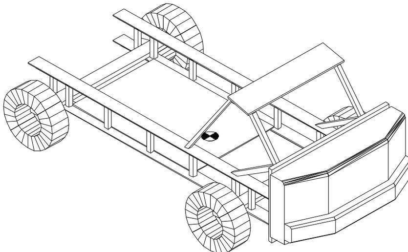
The deformable element has a width of 1,676 mm, a height of 759 mm, and a ground clearance of 379 mm when mounted on the test cart (Figure 3). Detailed information on the IIHS barrier development and evaluation testing has been documented previously (Arbelaez et al., 2002). The IIHS deformable barrier design and performance criteria are documented in the *Side Impact Moving Deformable Barrier Specification* (IIHS, 2007).
