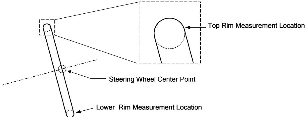
Enter the coordinates of the steering wheel points into the appropriate cells of the *CMM Data* worksheet. The steering wheel center point will automatically be calculated from the spatial average of the points recorded in steps 2.3.1 and 2.3.2.
