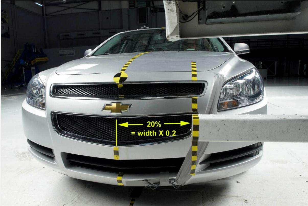
The striking vehicle is accelerated by the propulsion system until it reaches the test speed and then is released from the propulsion system approximately 25 cm before impact with the semitrailer. The onboard braking system, which applies the vehicle's service brakes on all four wheels, is activated 1.0 second after the vehicle is released from the propulsion system.
