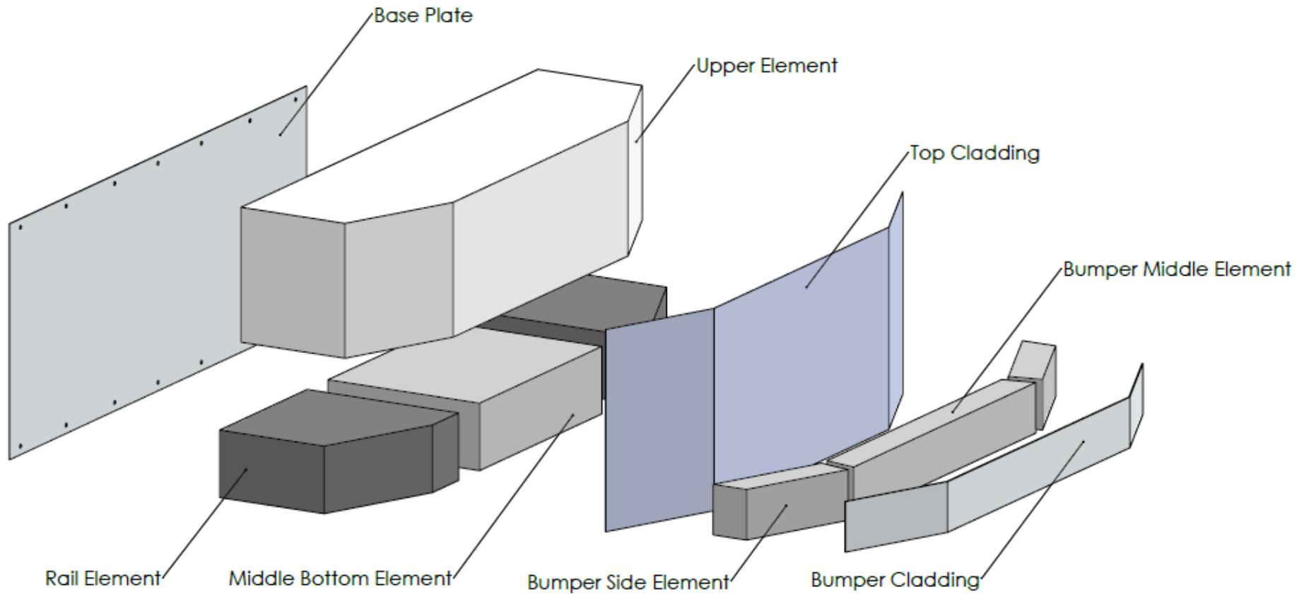
**Figure 2. General Assembly of the Main and Bumper Honeycomb Blocks**
