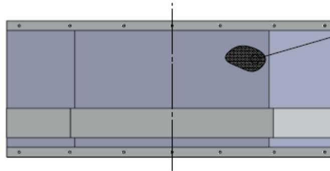
Detail showing ribbon orientation of honeycomb.
