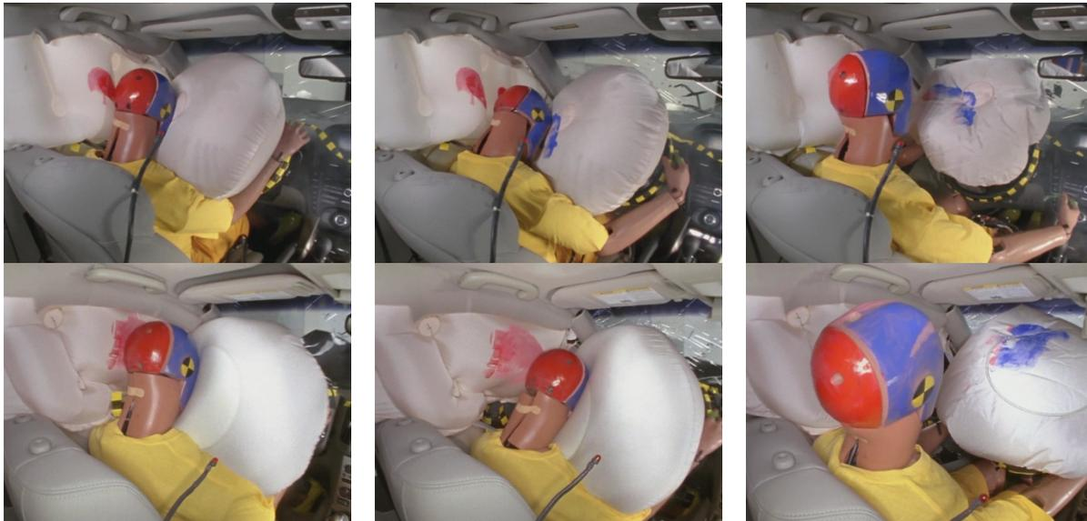
During both of these crashes, the heads loaded and remained engaged with the frontal airbags until rebound.
