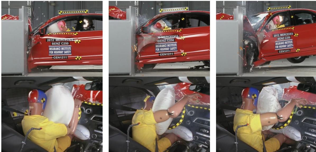
During the crash, the dummy's head loaded the frontal airbag but then rolled around it to the left side. There were no other countermeasures to prevent head contact with hard structures forward of the airbag.
