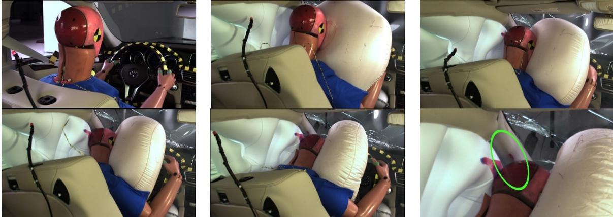
During the crash, the dummy's head loaded the frontal airbag but then rolled partly around it to the left side. The dummy's head contacted the a-pillar because there were no other countermeasures forward of the airbag.
