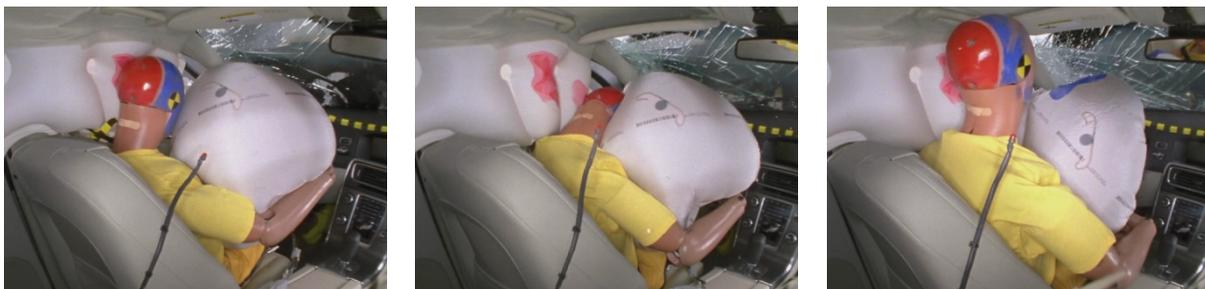
During the crash, the dummy's head briefly loaded the frontal airbag before sliding off the left into a gap between the frontal and side curtain airbags. The frontal airbag was narrow, and there were no other countermeasures to prevent head contact with hard structures forward of the airbag.
