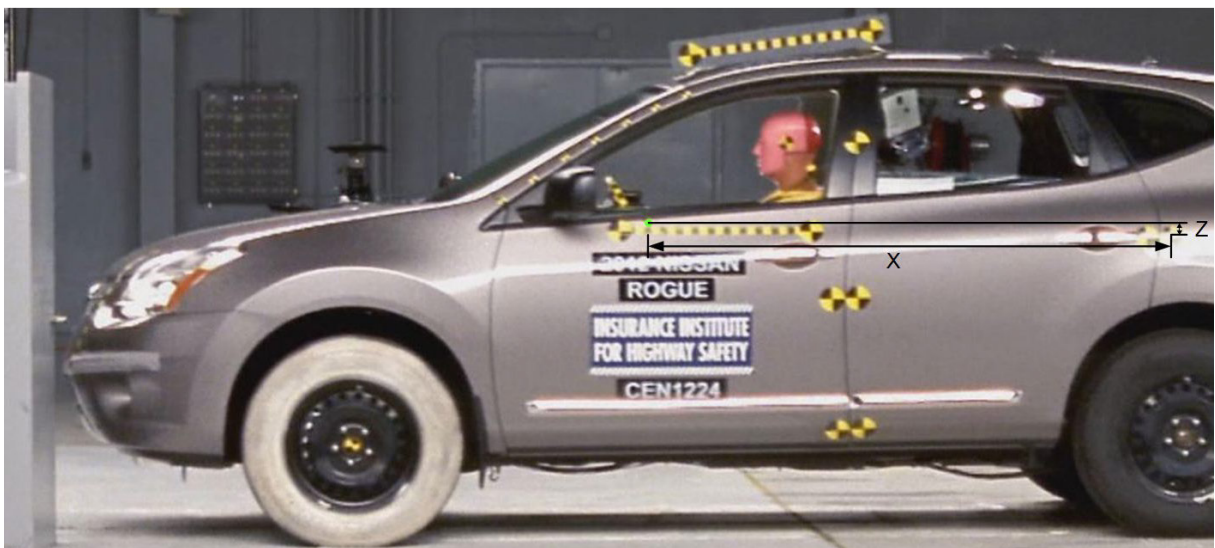
Figure B2 Distance between horizontal door targets (61 cm), all vehicles
