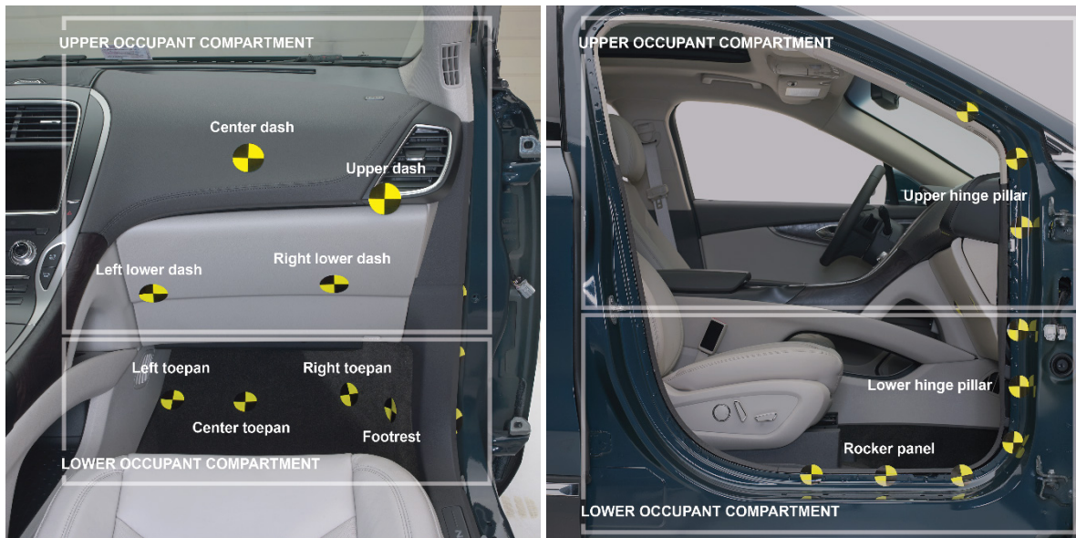
Figure D3 Locations for measuring vehicle intrusion — Passenger side
