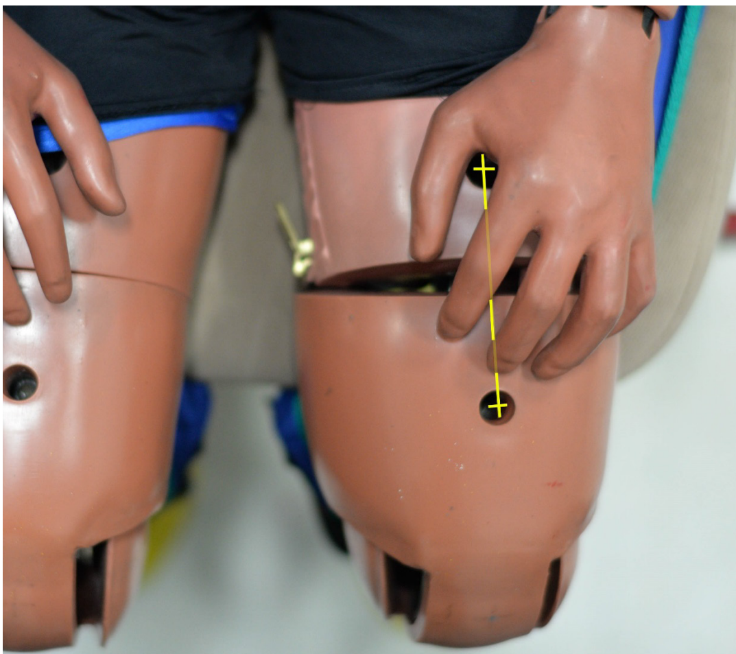
Figure D2 Dummy hand placement — Passenger side
