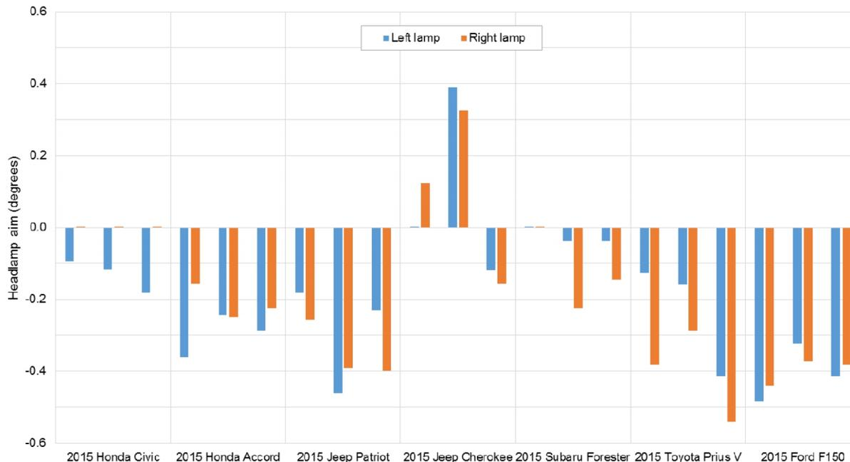
procedures during vehicle production, there are multiple reasons that some vehicle manufacturers may intentionally be aiming their headlamps at angles other than 0 degrees. To reflect their real-world performance, vehicles will be tested as received, with the headlamp aim unadjusted from its factory setting.
