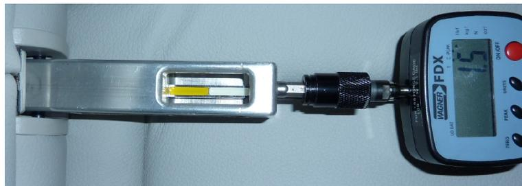
**Figure 7. Force tool slider fully engaged on anchor.**
