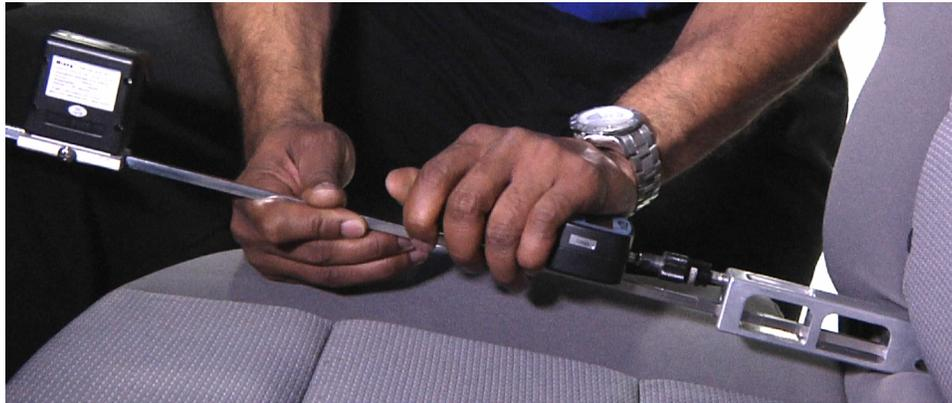
**Figure 6. Measuring lower anchor attachment force.**
