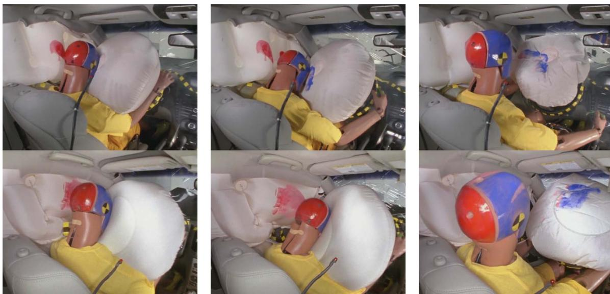
The dummy's movement in these tests was well controlled. The dummy's head loaded the frontal airbag and stayed in contact with the airbag within its original extended perimeter until the dummy rebounded in the rearward direction.
