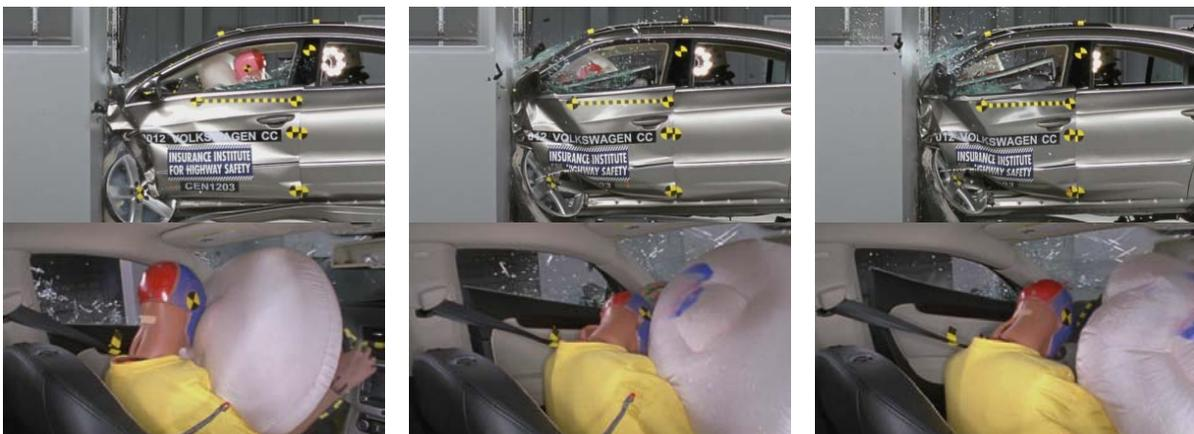
The dummy's head barely contacted the frontal airbag before sliding off the left side and undergoing additional forward excursion. There were no other countermeasures to prevent head contact with hard structures forward of the airbag.
