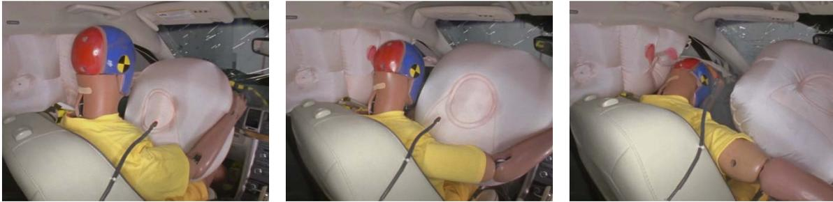
The dummy's head completely missed the frontal airbag, and there were no other countermeasures to prevent head contact with hard structures forward of the airbag.
