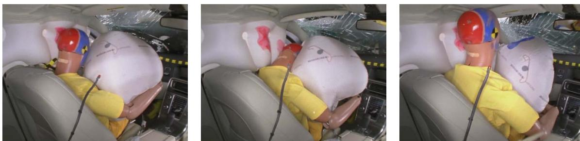
The dummy's head contacted the frontal airbag but slid left into a gap providing no support for the head. This gap mainly was due to the narrow, asymmetric frontal airbag. There were no other countermeasures to prevent head contact with hard structures forward of the airbag.
