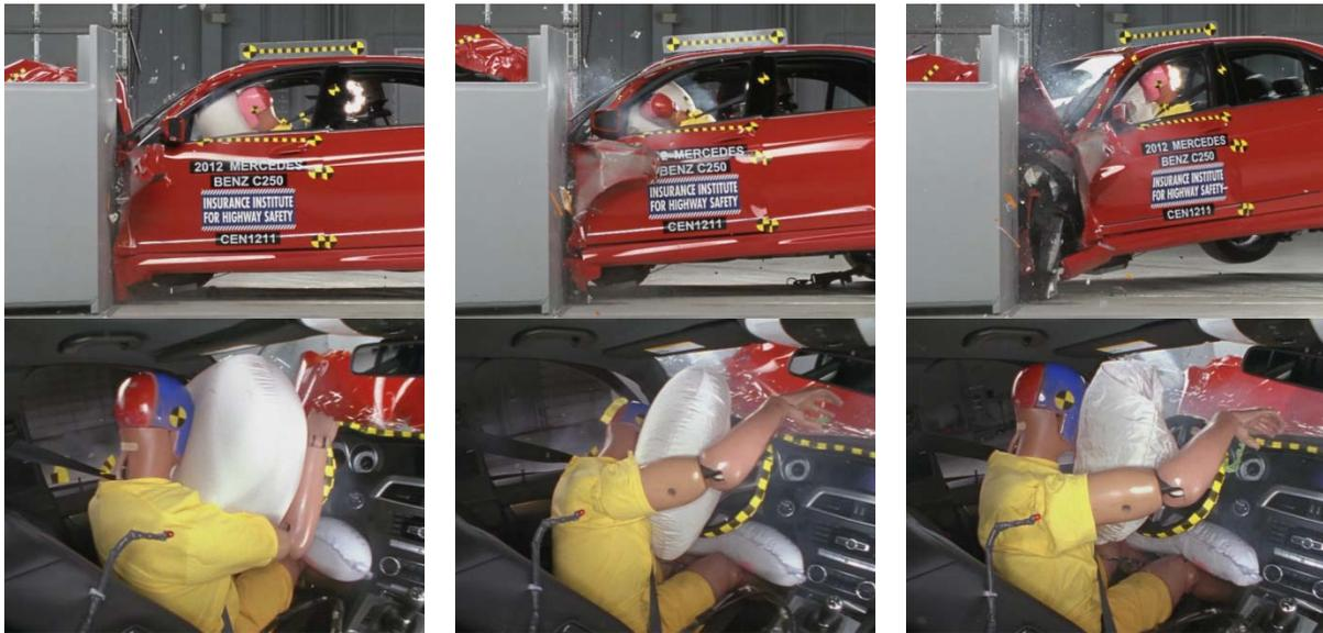
The airbag provided significant support to the head early in the crash, but the dummy continued to move laterally outside of the original extended perimeter of the airbag, and there was little airbag volume between the dummy's head and interior structures. The dummy contacted the roof rail during rebound. There were no other countermeasures to prevent head contact with hard structures forward of the airbag.
