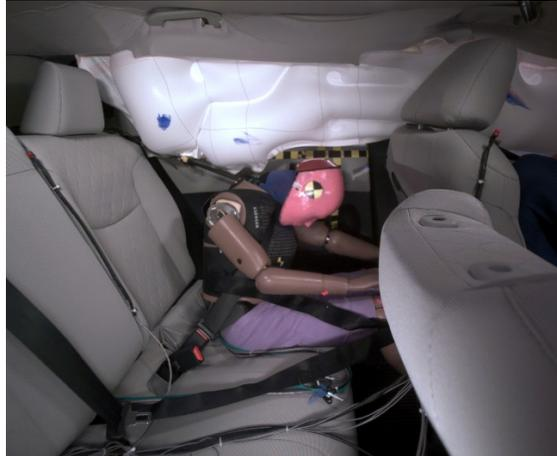
**Figure 3b.** At maximum forward excursion, a judgment on how far the head has moved is made using these lines
