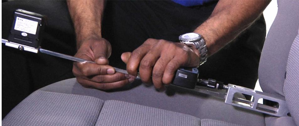
**Figure 6. Measuring lower anchor attachment force.**
