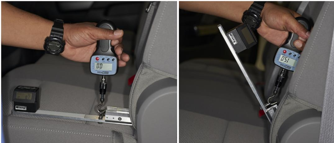
**Figure 9. Measuring lower anchor clearance angle.**
