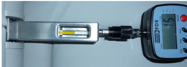
**Figure 7. Force tool slider fully engaged on anchor.**
