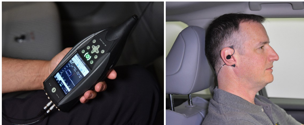
Figure 1. Data recorder and microphone location
