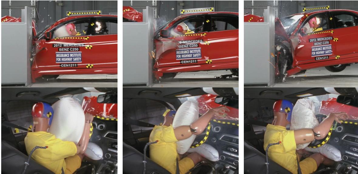
During the crash, the dummy's head loaded the frontal airbag but then rolled around it to the left side. There were no other countermeasures to prevent head contact with hard structures forward of the airbag.
