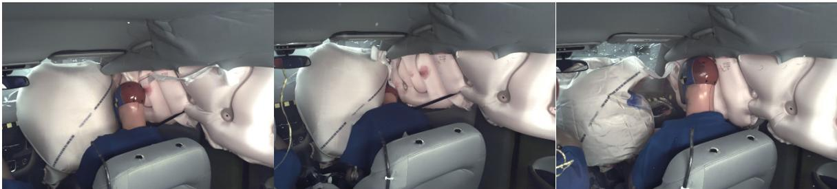
During the crash, the dummy's head barely contacted the frontal airbag before sliding off the right side of the airbag into the gap between the frontal and side curtain airbags. There were no other countermeasures to prevent head contact with hard structures forward of the airbags.
