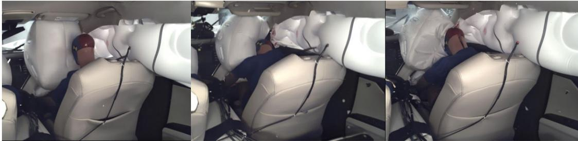
During this crash, the dummy's head briefly loaded the right side of the frontal airbag before contacting the dash through the airbag, though the side curtain helped keep the head on the frontal airbag.
