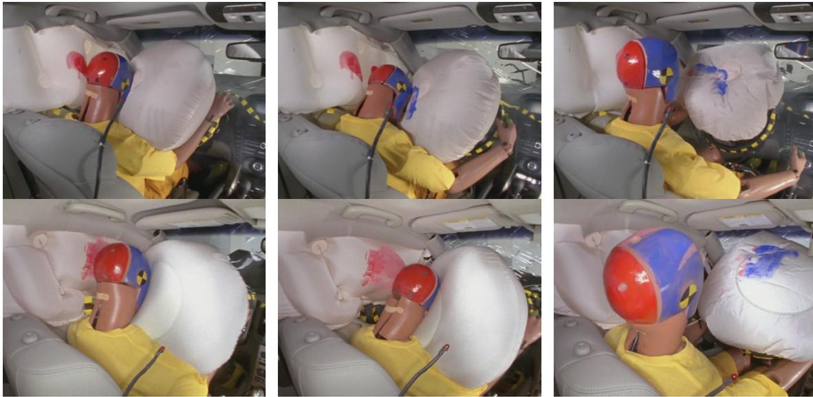
During both of these crashes, the heads loaded and remained engaged with the frontal airbags until rebound.
