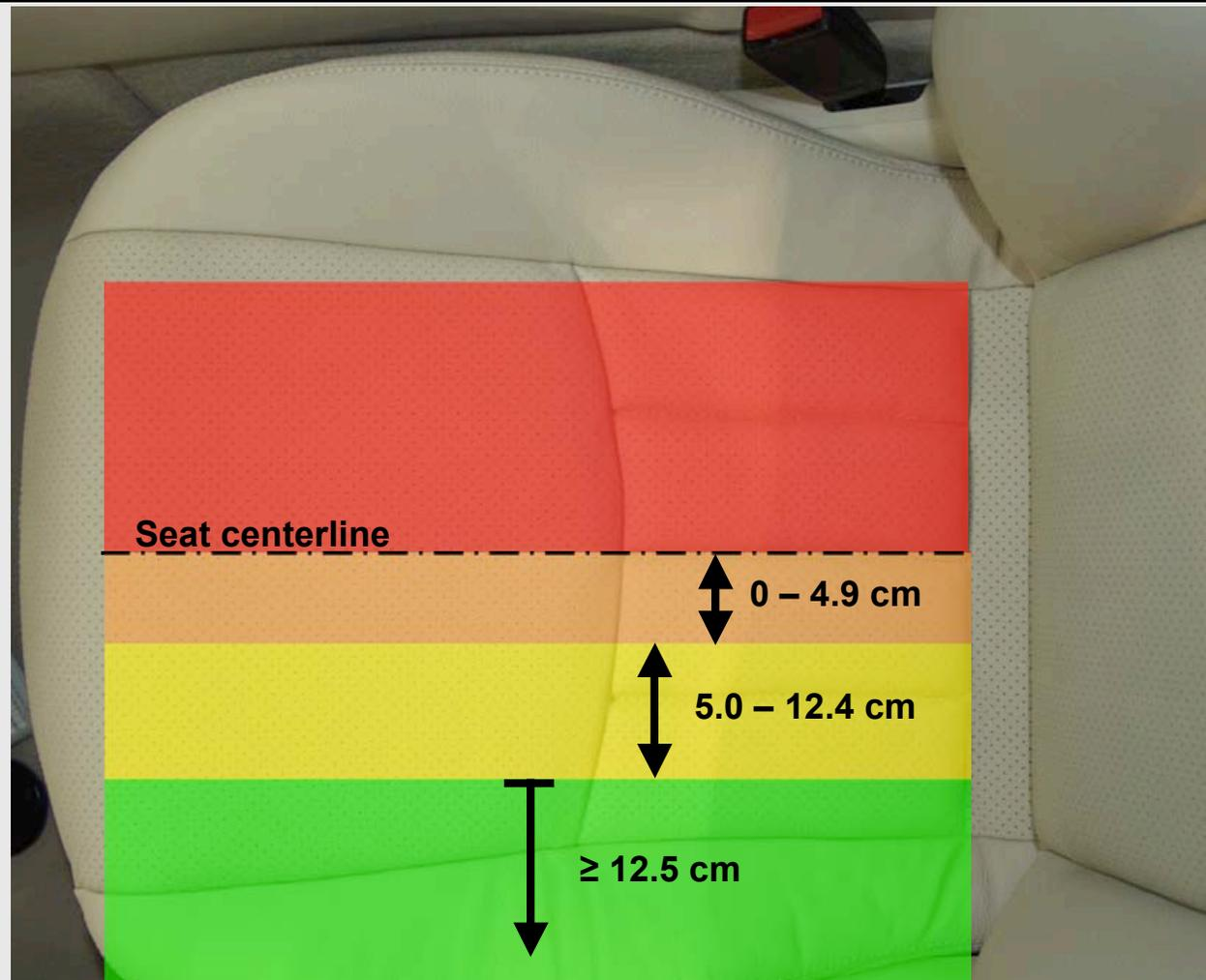
Good: B-pillar point of maximum intrusion is  $\geq 12.5$  cm from seat centerline
