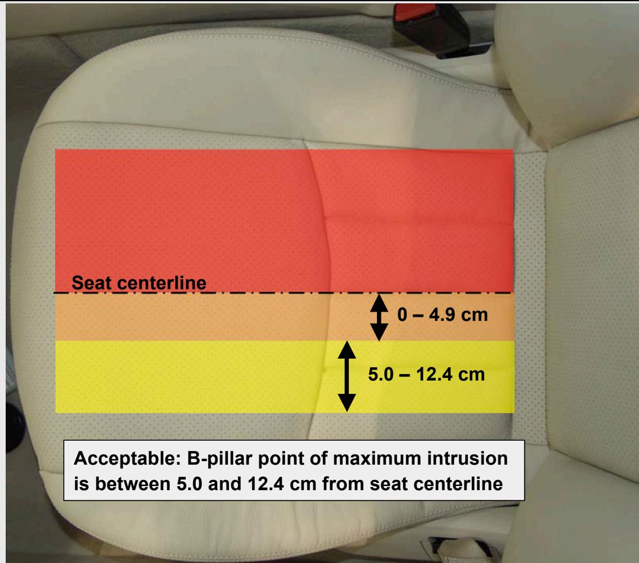
**Acceptable: B-pillar point of maximum intrusion is between 5.0 and 12.4 cm from seat centerline**
