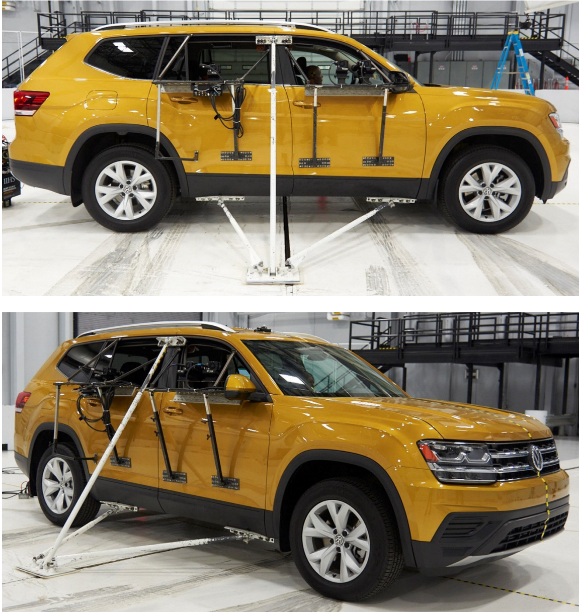
Figure 5 Antiroll device for tests of midsize and large SUVs, pickups, and passenger vans
