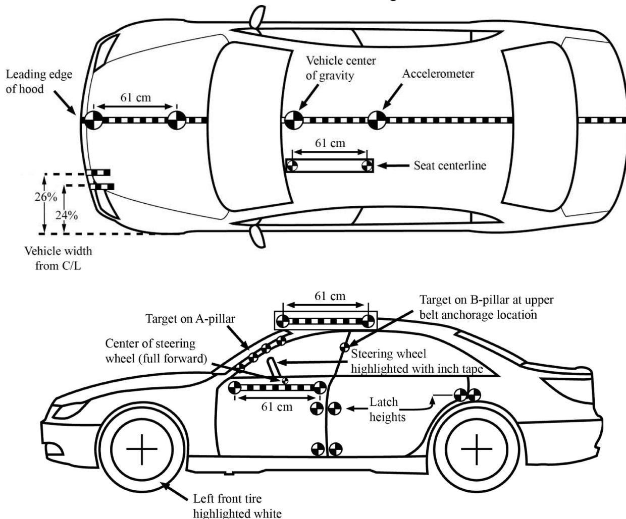
steering wheel center in the longitudinal direction. To determine vehicle alignment with the barrier at impact, inch tape is placed at 24 and 26 percent of vehicle width. The steering wheel and the leading edge of the dash are highlighted with inch tape, and the left front tire is highlighted with white paint.
