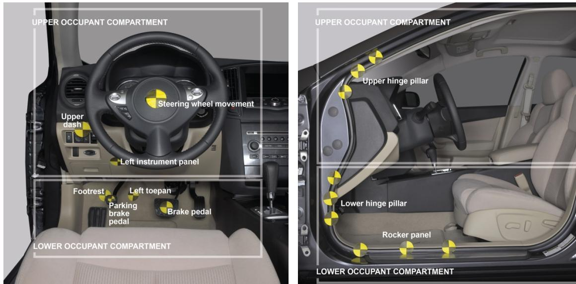
**Left lower instrument panel (one point):** The left lower instrument panel (knee bolster) lateral coordinates are defined by subtracting 15 cm from the steering column reference lateral coordinate, respectively. The vertical coordinate is defined as 45 cm above the height of the floor (without floor mats). If the panel or knee bolster loosens or breaks away in the crash, the postcrash measurements are taken by pressing and holding the panel against the underlying structure.
