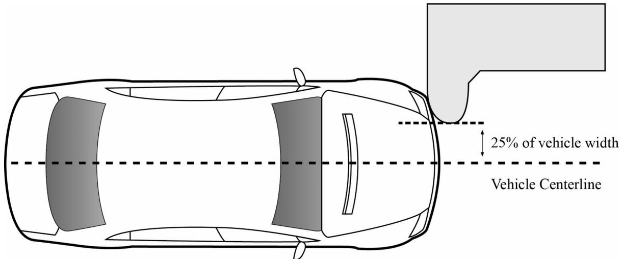
The vehicle is accelerated by the propulsion system at an average of 0.3 g until it reaches the test speed and then is released from the propulsion system approximately 25 cm before the barrier. The onboard braking system, which applies the vehicle's service brakes on the rear wheels, is activated 1 second after the vehicle is released from the propulsion system.
