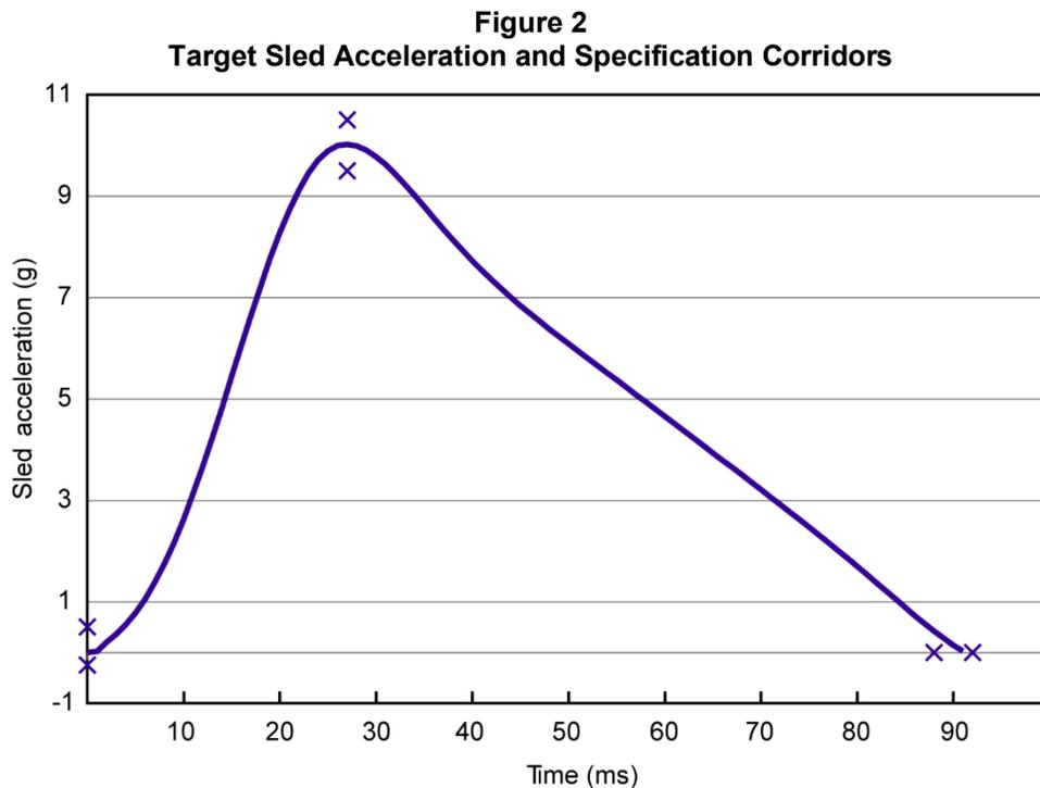
\* This typically is done by subtracting the average value of approximately 100 preimpact data points from each acceleration measurement during the test.
