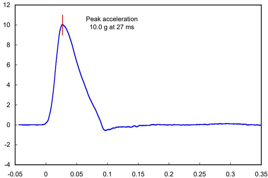
Step 4. Filter sled acceleration data to CFC 180. Integrate from the last time the acceleration passes through zero at the beginning of the trace until the first time the acceleration passes through zero at the end of the trace.
