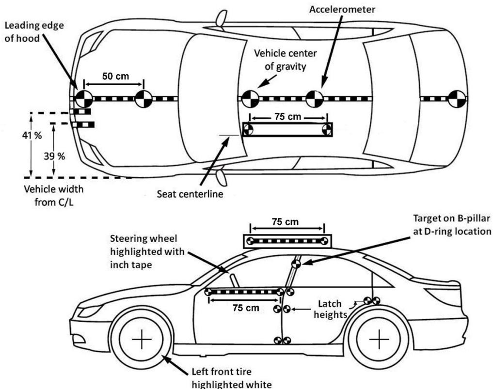
The interior surfaces of the vehicle are also trimmed with tape and photographic targets to facilitate analysis of the high-speed digital video (Figure 5).
