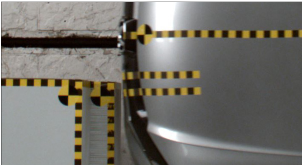
Figure 7 Determining vehicle overlap — Video screen shot
