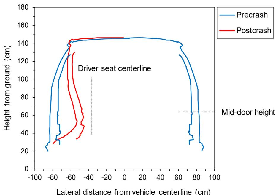
Seat belt retractors are included in the precrash measures if they are located within the vertical measurement range of the interior B-pillar (Figure 8). Only the structural components of the retractor, or crash tensioner, are measured (i.e., metal bracketry and bolts), not the seat belt webbing spool.
