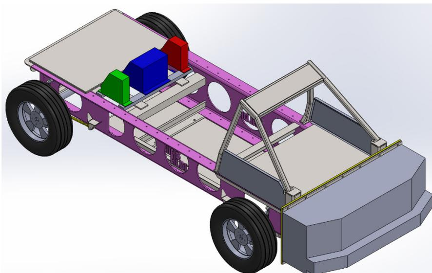
The deformable element has a width of 1,700 mm, a height of 600 mm, and a ground clearance of 350 mm  $\pm$  0.5 cm when mounted on the test cart (Figure 3).
